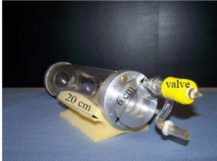
Figure 4.6: Overview of the target cell used in the photon beam.
