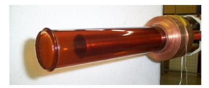
Figure 4.11: Liquid hydrogen target cell [105].
