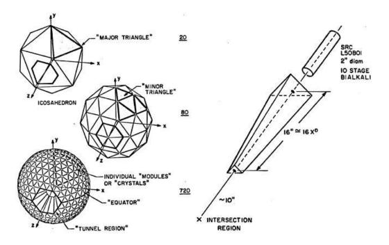
Figure 4.14: Sketch of the geometry of CB and of its crystals [108].
