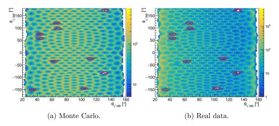
Figure 7.13: Angular distribution in the CB of simulated and real Compton scattering events in the left and right panel, respectively. The red ellipses shows the ten problematic CB channels.
