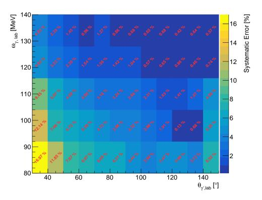
Figure 8.12: Systematic errors due to the background contamination as a function of the beam energy  $\omega_{\gamma}$  and the scattering angle  $\theta_{\gamma'}$ . They are calculated as the relative empty target contribution to the full target sample scaled by a normalization factor. This factor is determined such that the background peak in the empty target fully describe the one in the full target.
