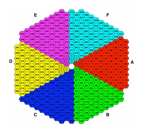
Figure 4.20: Scheme of the TAPS crystal distribution. In the first two innermost rings each  $BaF_2$  crystal is replaced by four  $PbWO_4$  crystals. The different colors correspond to different sections of electronic acquisition system [112].
