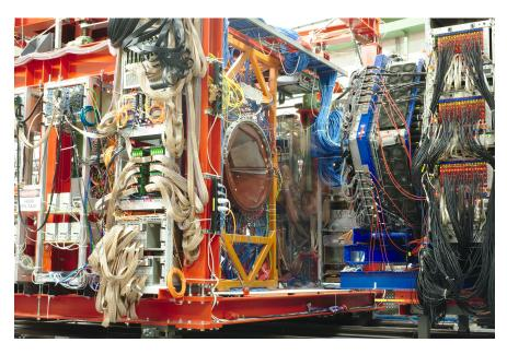
Figure 4.13: Crystal Ball detector installed in the A2 Collaboration experimental hall. The photon beam comes from the left, outside the figure, and hits the target in the center of the CB. TAPS, covering the forward region, is also visible on the right. Figure taken from Ref. [106].
