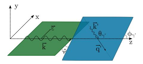
Figure 9.1: Scheme of the photon polarization and reaction scattering planes. The former, in green, is defined by the incoming photon momentum  $\vec{k}$  and the polarization vector  $\vec{\epsilon}$ . The latter, in blue, is given by the scattered photon and the recoil proton momenta  $\vec{k'}$  and  $\vec{q'}$ , respectively. Adapted from Ref. [97]
