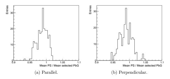
Figure 6.8: Distribution of the pair spectrometer scaling factor to correct the tagging efficiency magnitude for a sample of the total dataset obtained with the two orientations of the diamond radiator.
