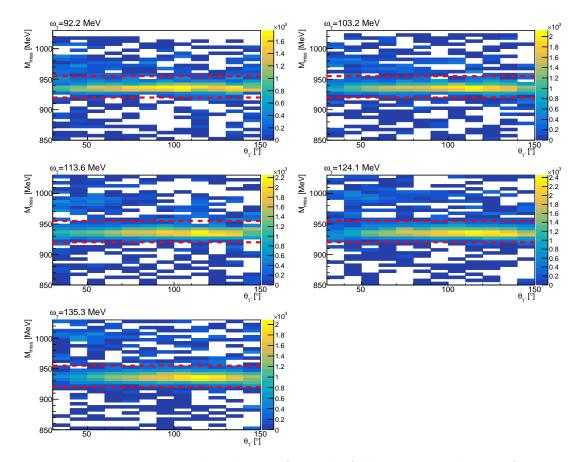
Figure 8.9: Missing mass distribution from the full target sample as a function of the scattering angle  $\theta_{\gamma'}$  for the five different bins in beam energy, after the subtraction of the empty target contribution. The red dotted lines show the missing mass cuts applied in the analysis. Some remaining background is still visible for  $\theta_{\gamma'} < 50^{\circ}$  and  $M_{miss} > 960$  MeV.
