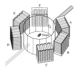
Figure 3.1: TAPS apparatus used for the Olmos de Léon *et al.* measurement. The photon beam enters from the top-right corner, between blacks F and A. The figure is reproduced from Ref. [67].
