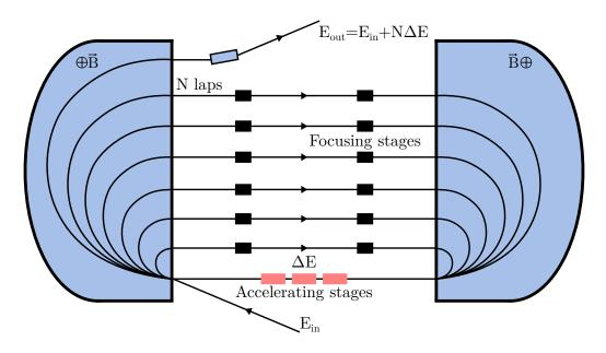
Figure 4.3: Scheme of a racetrack microtron (RTM).
