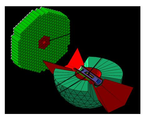
Figure 4.12: Sketch of the detector system in the A2 Collaboration hall. The photon beam comes from lower right and hits the target at the center of the Crystal Ball (CB). The different detectors are visible: the Particle Identification Detector (PID), two Multi Wire Proportional Chambers (MWPCs) and the CB, around the target from the innermost, and TAPS in the upper left corner, covering the forward region.
