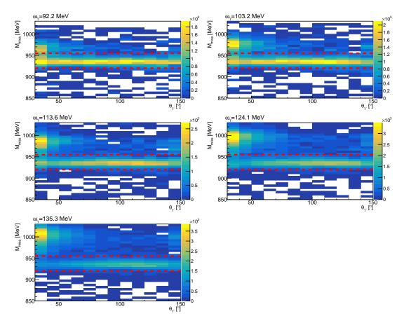
Figure 8.8: Missing mass distribution from the full target sample as a function of the scattering angle  $\theta_{\gamma'}$  for the five different bins in beam energy. The red dotted lines show the missing mass cuts applied in the analysis. The background peak is clearly visible for  $\theta_{\gamma'} < 50^{\circ}$  and  $M_{miss} > 960$  MeV.
