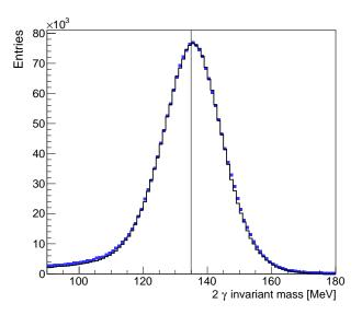
Figure 7.12: Example of 2- $\gamma$  invariant mass distribution for a given  $\theta_{\gamma'}$  bin. The simulated distribution in black is compared with the empty target subtracted distribution in blue. The nice agreement among the two distributions demonstrates an appropriate Monte Carlo calibration and smearing.
