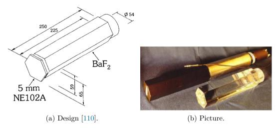
Figure 4.19: (a) Design and (b) picture of a single  $BaF_2$  crystal.
