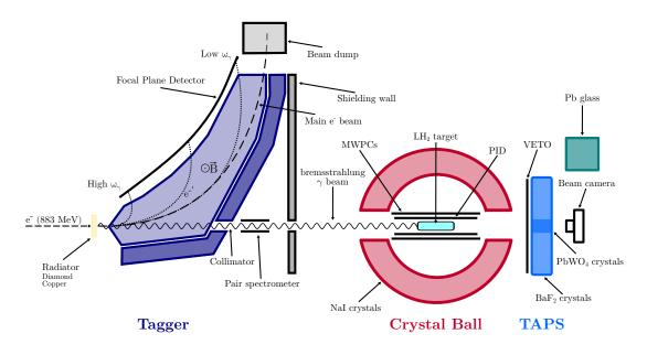
Figure 4.1: Overview of the experimental apparatus in the A2 Collaboration hall. The electron beam comes from the left and hits the radiator producing bremsstrahlung photons. Electrons are bent by the tagger spectrometer in blue, while the photon beam passes through a collimator and hits the  $LH_2$  target. The particles in the final state are detected by the Crystal Ball and the TAPS apparatuses in red and light blue, respectively.
