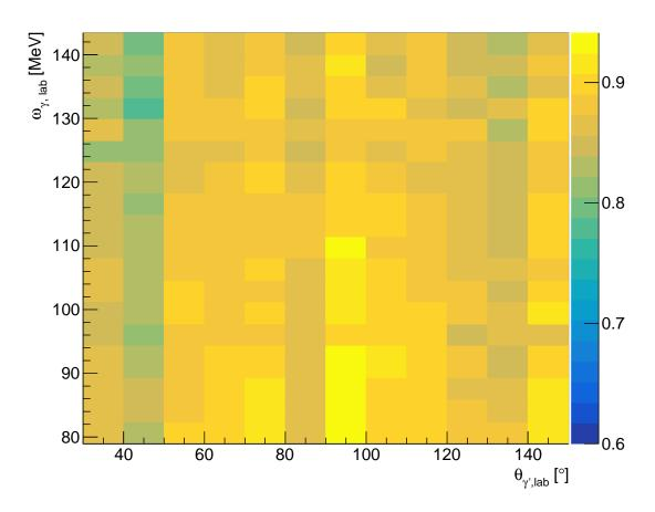
Figure 7.14: Compton scattering detection and reconstruction efficiency as a function of the photon beam energy  $\omega_{\gamma}$  and the scattering angle  $\theta_{\gamma'}$ . The drop in efficiency visible at  $\theta_{\gamma'} = 45^{\circ}$  is due the missing channels in the CB reported in Fig. 7.13.
