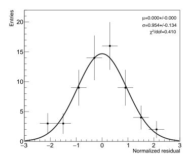
Figure 8.13: Normalized residual for the unpolarized Compton scattering crosssection obtained using March 2018 data with respect to the results obtained using July 2018 data. A Gaussian fit was also performed (black line), and the results are reported on the right.
