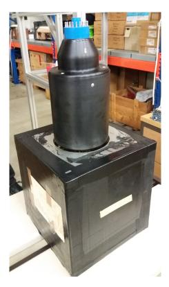
Figure 4.21: Picture of the lead glass detector during maintenance work [113].
