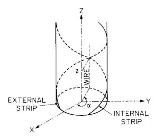
Figure 4.18: Coordinate system used in the MWPCs analysis. The photon beam comes from the bottom and travels along the z-axis. Within each chamber the azimuthal  $\alpha$  and longitudinal zeta coordinates are evaluated from the charge distribution induced on the cathode strips. Since each pair of inner and outer strips cross each other twice, the position of the hit wires is needed to resolve the ambiguity. Figure taken from Ref. [71].
