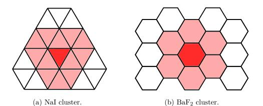
Figure 5.1: Cluster structure of (a) Crystal Ball and (b) TAPS. The central crystal is colored in red, together with the nearest neighbors — 12 and 6 for CB and TAPS, respectively — colored in pink.
