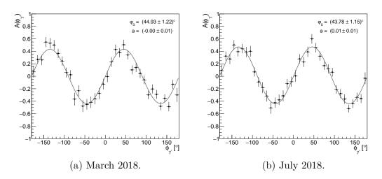
Figure 9.3: Extraction of  $\varphi_0$  from the  $A(\phi_{\gamma'})$  distribution separated for the two main beamtimes. The gray curves are the fit functions defined in Eq. (9.3). The values of both  $\varphi_0$  and a are reported in the canvas.
