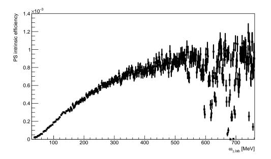
Figure 6.5: Average intrinsic pair spectrometer efficiency as function of the photon energy.
