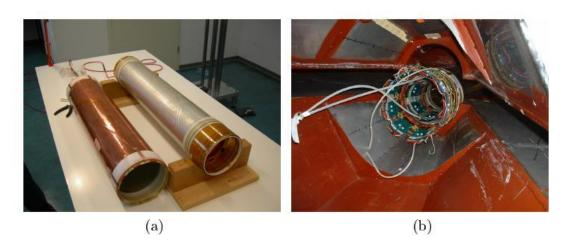
Figure 4.17: (a) Picture of the inner and outer cathodes during repair of the MWPCs. (b) Picture of the MWPCs installed inside the CB.
