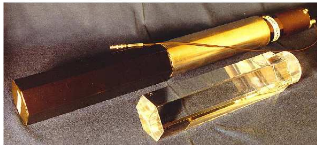
Figure 3.10: Each individual TAPS \text{BaF}_2 detector consists of a hexagonally shaped crystal tube of 25 cm in length with a 2.5 cm cylindrical end connected directly to the photomultiplier tube.
