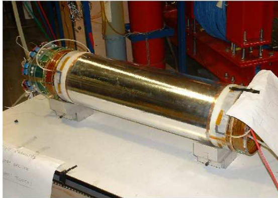
Figure 3.9: The Multiwire Proportional Chamber before inserting it into its position within the CB.
