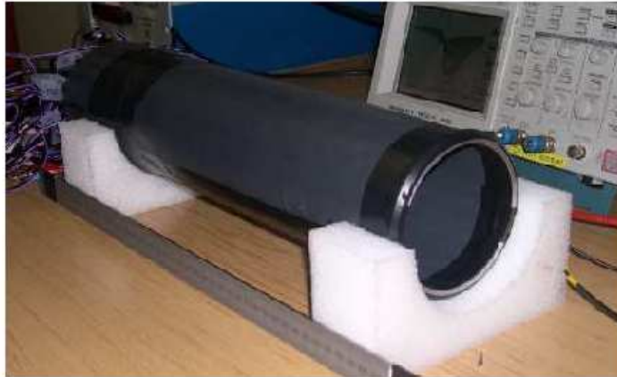
Figure 3.8: The PID before inserting it into position within the CB.
