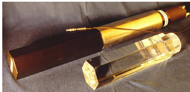
(b) A Barium Fluoride crystal and assembled detector element
