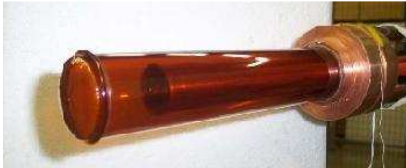
Figure 3.9: The Liquid Hydrogen Target
