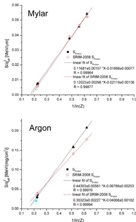
**Fig. 1:** Stopping force dependence on  $Z$ . Stopping force values from H. Paul [5] (full triangles) and from our measurements (full circles) in Mylar (upper graph) and gaseous argon (lower graph). The empty circles are simulated SRIM-2008 values. The lines (black for experimental values, red for SRIM-2008 values) represent linear regressions showing the dependence of the STF from the atomic number  $Z$ .
