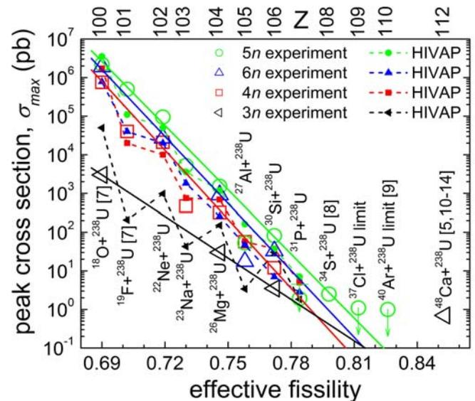
**Figure 1:**  $\sigma_{max}$  (open symbols) as a function of effective fissility [16]. Heavy straight lines (top to bottom) are exponential fits to even- $Z$   $\sigma_{max}$  for the 5n, 6n, 4n, and 3n exit channels. Filled symbols connected by dashed lines are results of HIVAP calculations [15]. References
