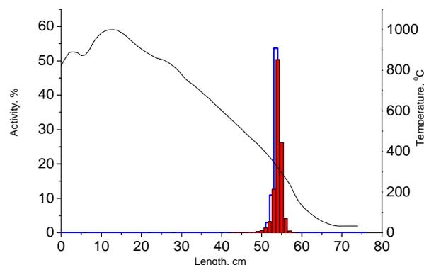
**Figure 2:** Thermochromatogram of  $^{113\text{m}}\text{In}$  on quartz surface (red filled area – experimental results, blue line – results of Monte-Carlo simulations).
