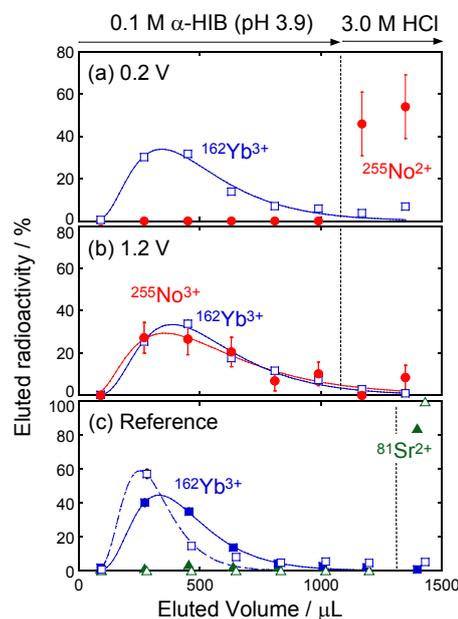
**Figure 1:** Elution behavior of  $^{255}\text{No}$  and  $^{162}\text{Yb}$  at the applied potentials of (a) 0.2 V and (b) 1.2 V. (c) Elution of the typical trivalent  $^{162}\text{Yb}^{3+}$  and the divalent  $^{81}\text{Sr}^{2+}$  in the reference experiment: close symbols at 1.2 V, open symbols at 0.2 V.
