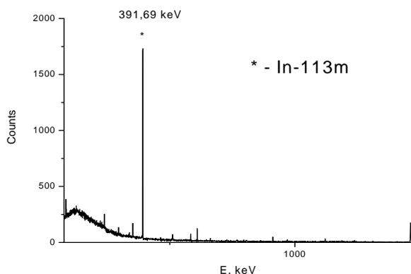
**Figure 1:** Gamma spectrum of  $^{113\text{m}}\text{In}$  eluted from a Sn isotope generator
