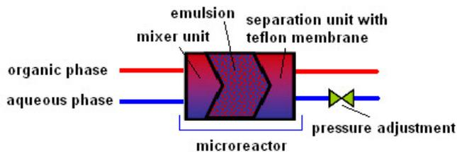
Figure 1. Schematic setup for experiments with MicroSISAK
