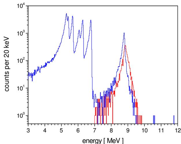
**Fig. 2:**  $\alpha$ -spectra of  $^{232}\text{U}$  and its descendents using the non-optimized PURECOLD spectroscopic system. Detected pile-up events are shown in red and the remaining events considered as purified alpha spectrum in blue.
