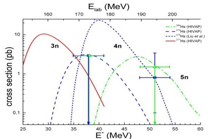
Figure 2: Production cross sections and limits measured for the reaction  $^{238}\text{U}(^{36}\text{S}, 3-5n)^{269-271}\text{Hs}$  in comparison with HIVAP calculations and calculations from [4]. Quadrates correspond to  $^{270}\text{Hs}$  ( $4n$  channel) and triangles correspond to  $^{269}\text{Hs}$  ( $5n$  channel)
