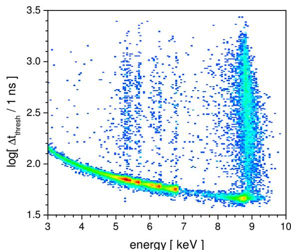
**Fig. 1:** Time difference between passing the first and 10<sup>th</sup> threshold versus  $\alpha$ -particle energy. A gap from 55 ns to 75 ns separates the true  $\alpha$ -events of  $^{212}\text{Po}$  from the  $\beta$ - $\alpha$  pile-up events of the decay of  $^{212}\text{Bi}$  and  $^{212}\text{Po}$ .
