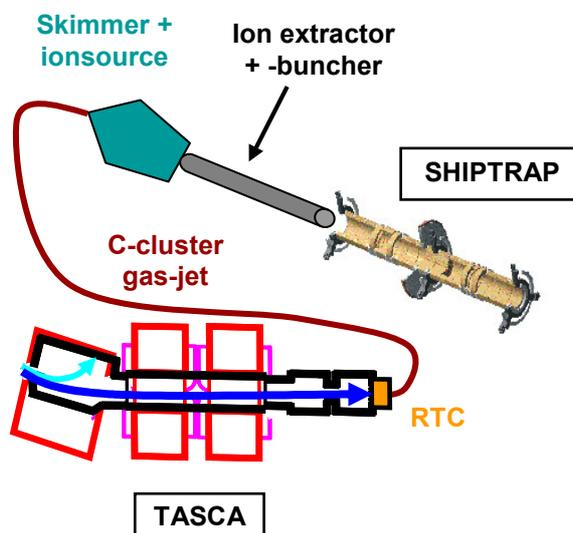
**Figure 1:** Coupling of TASCA and SHIPTRAP with a C-cluster gas-jet, a skimmer-unit and a subsequent ion source.
