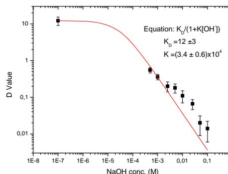
**Figure 1:** Distribution ratio of OsO<sub>4</sub> between NaOH solution and toluene vs. concentration of NaOH, obtained using the SISAK system in Oslo. The solid line shows the fitting of the result with equation (4).
