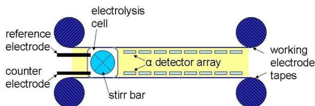
Figure 2: Schematic drawing of ELCH with the electrolysis cell (left) and the working electrode tapes stepped in front of an  $\alpha$ -detector array.
