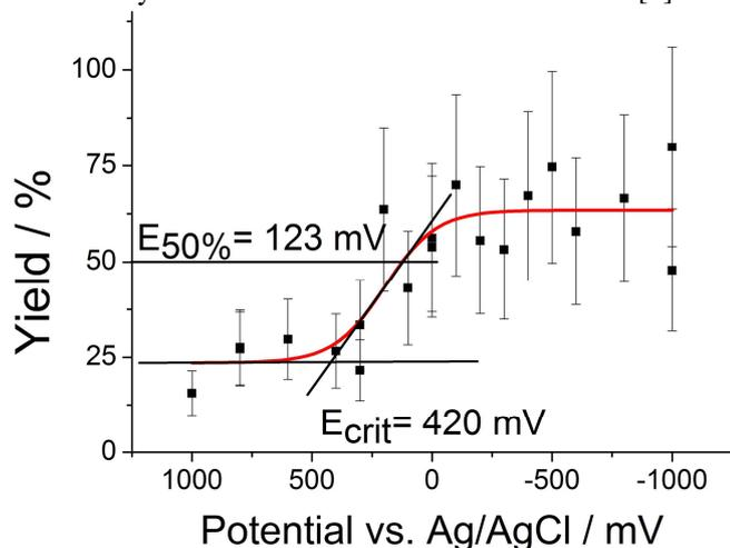
Figure 1: Deposition yield of Os on Pd electrodes as a function of the potential vs. Ag/AgCl.
