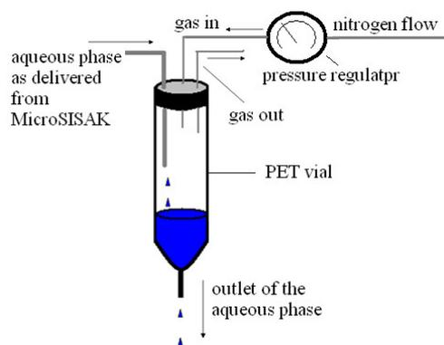
Figure 2: Scheme of the pressure regulation apparatus
