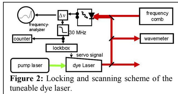
**Figure 2:** Locking and scanning scheme of the tuneable dye laser.
