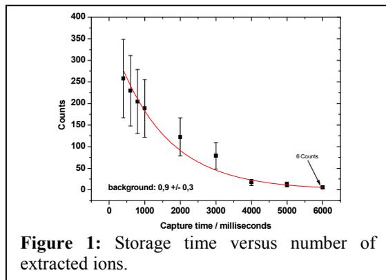
**Figure 1:** Storage time versus number of extracted ions.
