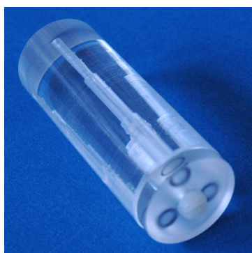
Fig. 1: Plexiglas phantom with 3 drills of 2, 3 and 4 mm in diameter, each.
