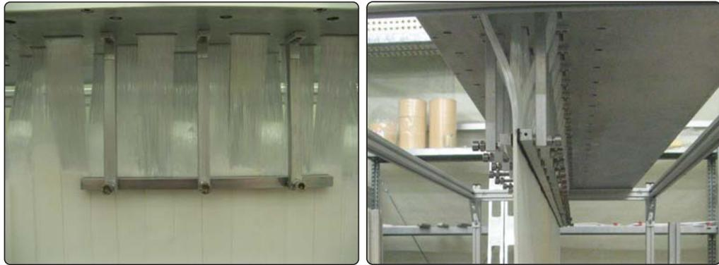
**Figure A.2:** Left. Photography of the crimping tool to keep the verticality of the fiber plane. Right. Side photography of the fiber plane showing how the crimping tool fits the plane.
