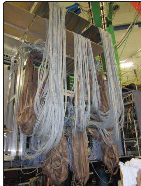
(d) Photography of the front-end electronics of the fiber detector hodoscope.
