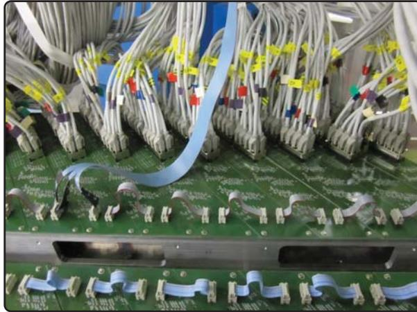
(b) Photography in detail of the triple boards with the signal cables already placed and the flat cables between the triple boards to power and control the HV bases of the MaPMT. The long blue flat cable is the main power and control cable from the HVSyS512 module
