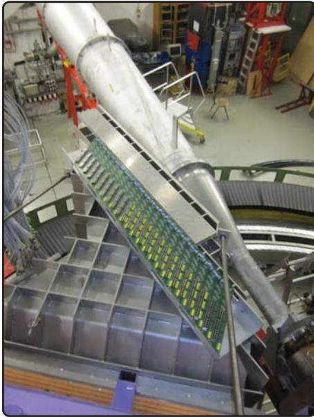
(a) Photography of one detector plane in the vacuum chamber without the cables.
