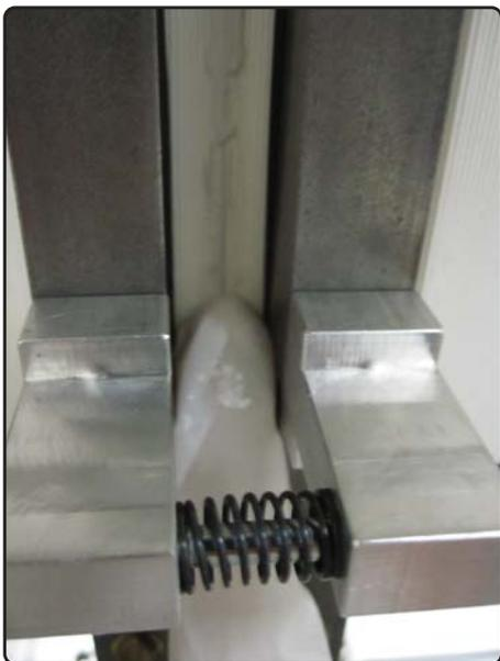
(c) Spread of the silicon layer applied in order to form a tiny layer.
