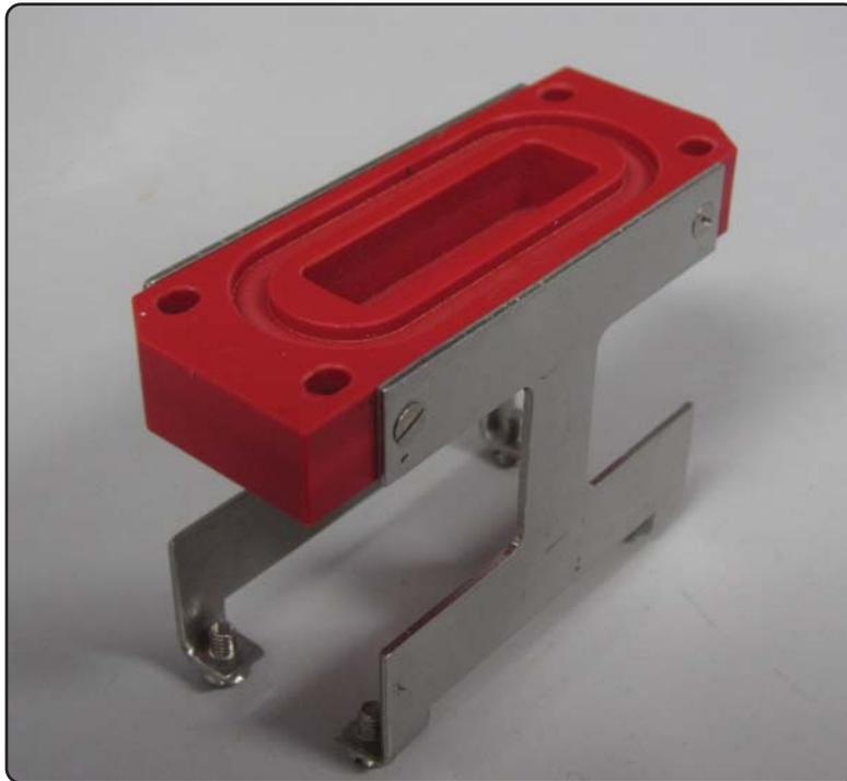
**Figure A.1:** Picture of the cookie with the clamping plates. It shows the groove for the O-ring for vacuum purposes. The hole in the middle is the place for glueing the fibers.
