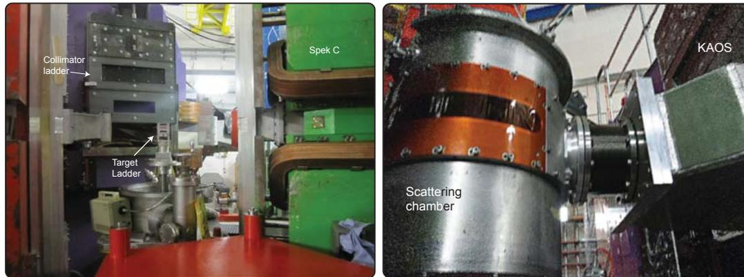
**Figure 1.7:** Left. Photo of the target position in the three spectrometer hall oriented from beam direction to beam dump. At left can be seen the collimator system at the entrance window of KAOS. In the center is the standard target ladder with different kind of solid state targets and at right the quadropole entrance of Spectrometer C. Right. Photo of the extension of the vacuum chamber of KAOS to the scattering chamber.
