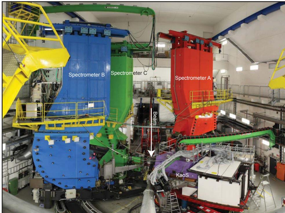
**Figure 1.4:** Panoramic view of the three spectrometers hall with the KAOS spectrometer showing the direction of the electron beam from MAMI (ca. 2009).
