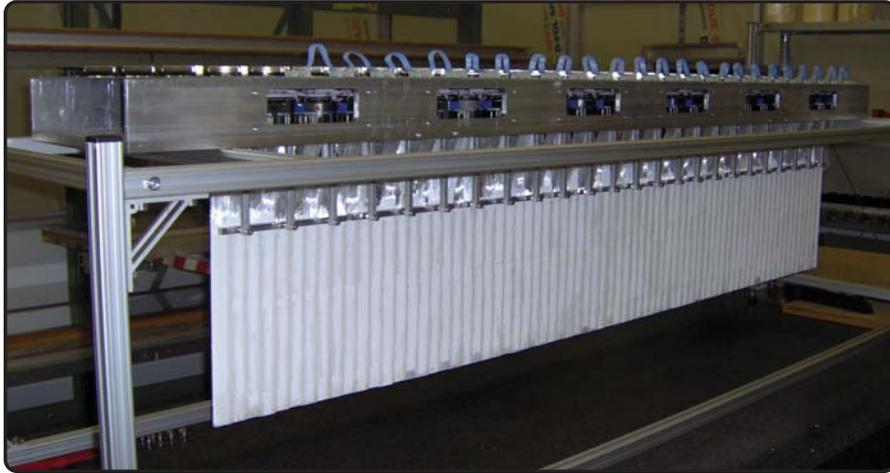
**Figure 2.44:** Photography of the fiber detector plane assembled in a supporting frame.
