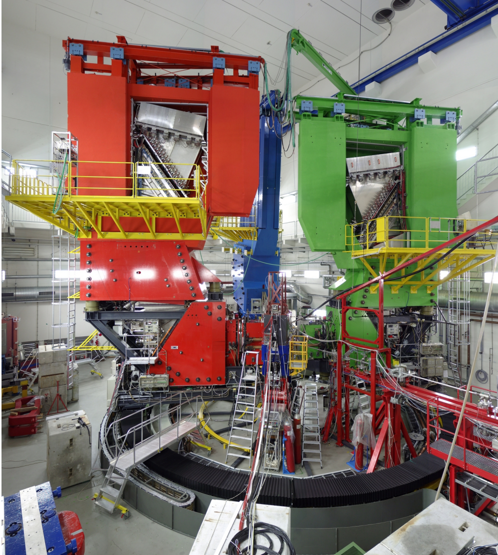
Figure 3.2: The A1 hall. The three big spectrometers A (red, left), B (blue, middle), C (green, right) are visible. The short orbit spectrometer SOS is positioned in front of the target, in the middle of the picture. The thin upstream beam-line pipe comes in from the right. As a dimension scale: A person is slightly taller than the concrete block on the lower left edge.
