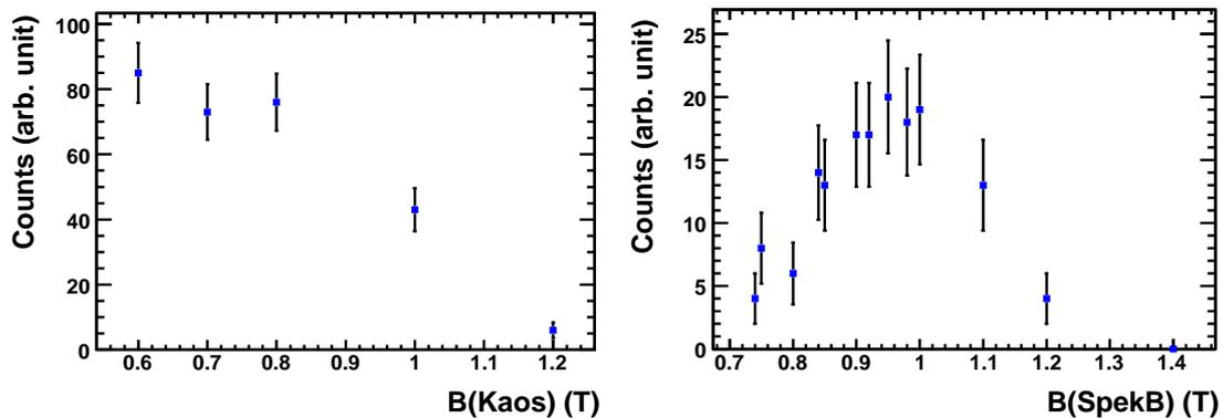
Figure 7: Left: count rate as a function of the magnetic field in KAOS at  $\vartheta = +30^\circ$ . An optimum field is found to be at  $B = 0.6$  T to tag  $K^+$  (momentum of 300 MeV/ $c$ ) from decayed  $\phi$ -meson. Right: count rate as a function of the magnetic field of SpekB at  $\vartheta_B = -15^\circ$ . The optimum field is found to be at  $B = 0.95$  T to tag  $K^-$  (momentum of 400 MeV/ $c$ ) from decayed  $\phi$ -meson.
