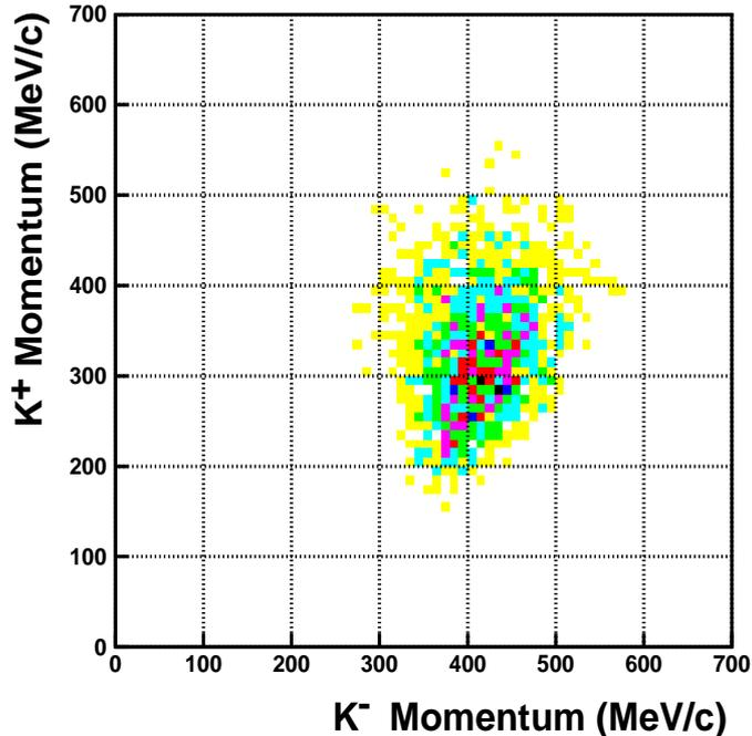
Figure 6: Momentum distribution for  $K^-$  and  $K^+$  after acceptance cut of KAOS and SpekB. The in-plane angles of KAOS and SpekB were set to  $+30^\circ$  and  $-25^\circ$ , respectively. Within the acceptance, the average  $K^+$  momentum was found to be 300 MeV/c while for  $K^-$  it was 400 MeV/c.
