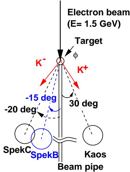
Figure 1: A possible set-up (top view) of the two spectrometers KAOS and SpekB or SpekC. Since the minimum angle of SpekC is  $\vartheta_{C,min} = -37^\circ$ , the configuration of  $\vartheta_C = -20^\circ$  is possible only if SpekB is moved to  $\vartheta_B \sim +90^\circ$  on the other side of the beam-pipe. The minimum angle of SpekB is  $\vartheta_{B,min} = -15.5^\circ$ .
