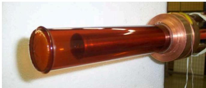
Figure 4.7: Inner Kapton cell of the liquid hydrogen,  $\text{LH}_2$ , target. The length of the target cell was  $100.0 \pm 1.0\text{ mm}$ , with a density of  $4.249 \times 10^{23}$  protons/ $\text{cm}^2$ . Reproduced from [55].
