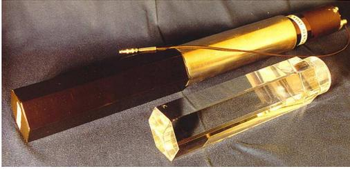
Figure 3.13: *Each TAPS element is made of a 25 cm BaF2 crystal corresponding to 12 radiation lengths. The main part of the crystal is hexagonal, with a 2.5 cm end cylinder connected directly to a photomultiplier for read-out.*
