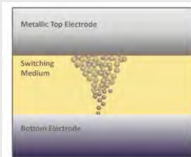
Figure 5: How it Works — In a switching media, nanoparticles form a conduction path between the top and bottom electrodes. from Crossbar
