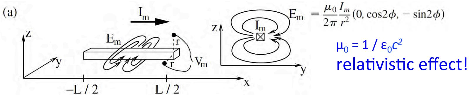
FIG. 3. (a) A current of magnetic dipole moment  $I_m$  produces an electric dipole field leading to a measurable voltage  $V_m$ . (b)
