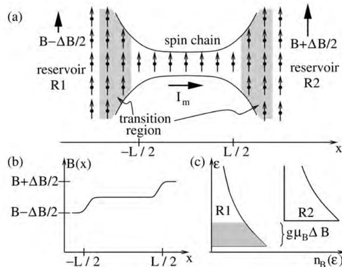
FIG. 1. (a) Proposed experimental setup for the measurement of a magnetization current  $I_m$ . (b) A magnetic field difference  $\Delta B$  between the two bulk systems gives rise to  $I_m = G\Delta B$ . (c)  $\Delta B$  shifts the Bose functions  $n_B(\epsilon)$  in the reservoirs R1 and R2. Magnons with energies  $\epsilon$  within the shaded region in R1 are not transmitted to R2.
