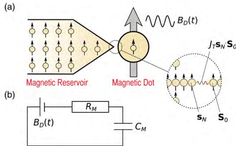
FIG. 1 (color online). (a) Schematic representation of the setup. The weakly coupled reservoir and dot are both modeled as 1D chains in this work. Parallel collections of such 1D chains are realized in bulk materials such as  $\text{SrCuO}_2$  (Ref. [30]) and  $\text{Cs}_2\text{CoCl}_4$  (Ref. [31]), as well as in ultracold atoms in optical lattices [32,33]. (b) Equivalent circuit representation of the setup; see Eq. (1) for the definition of  $R_M$  and  $C_M$ .
