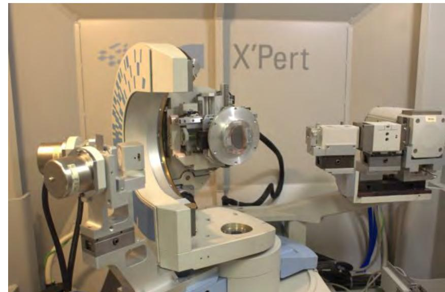
Phillips X-Pert high-resolution X-ray diffractometer
