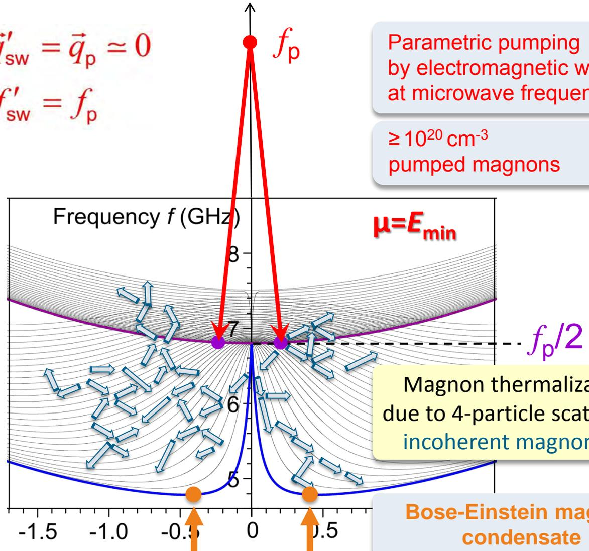
Magnon thermalization due to 4-particle scattering: incoherent magnon gas
