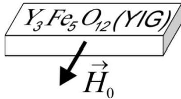
Thickness modes having a non-uniform harmonic distribution of dynamic magnetization along the film thickness
