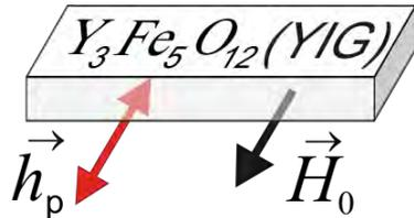
Parametric pumping by electromagnetic wave at microwave frequency
