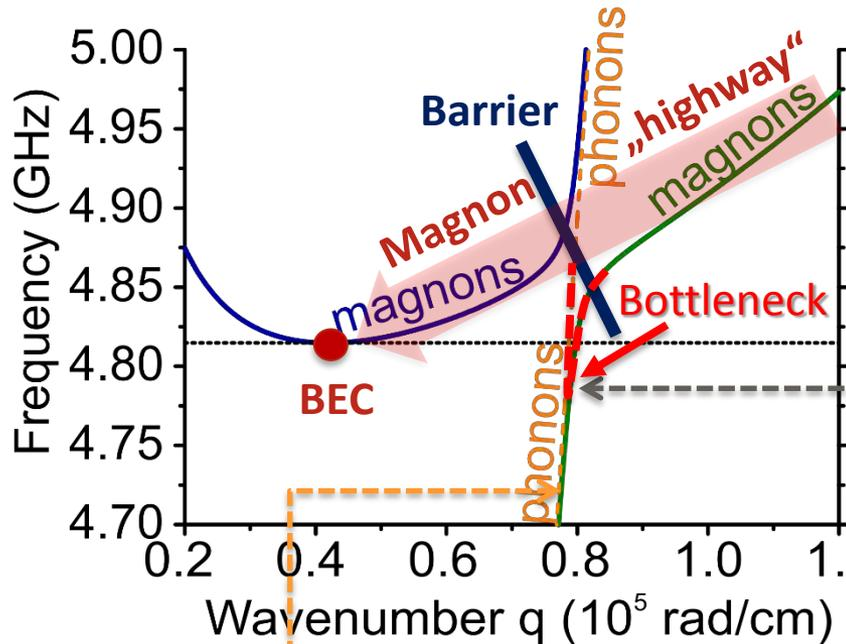
Magnon “highway” - current of magnons in a phase space to the BEC state
