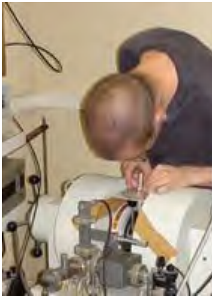
Student putting a macroscopic sample into a macroscopic ESR cavity
