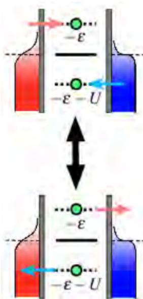
$$\kappa = \frac{J|_{I=0}}{\Delta T} = \frac{1}{T^2} \frac{\Gamma_L \Gamma_R}{\Gamma^2} \gamma_{p,\text{eq}} \left(\frac{U}{2}\right)^2 \delta n_{z,\text{eq}}^2 \delta n_{i,\text{eq}}^2$$
