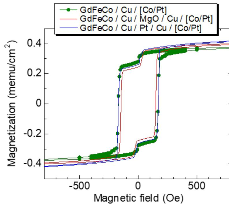
To test mechanism: MgO and Pt insertion in Cu
