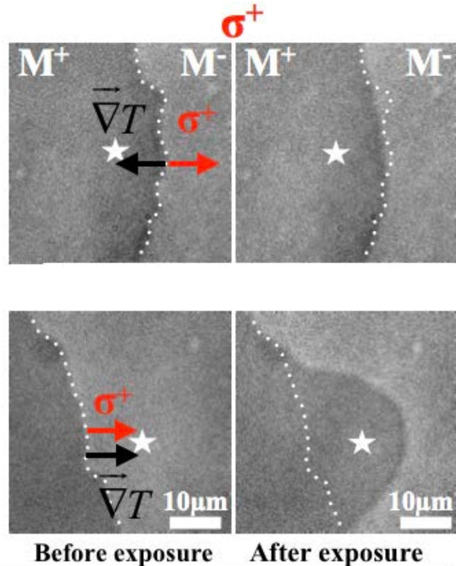
the **helicity effect** is *stronger* than the **temperature gradient**
