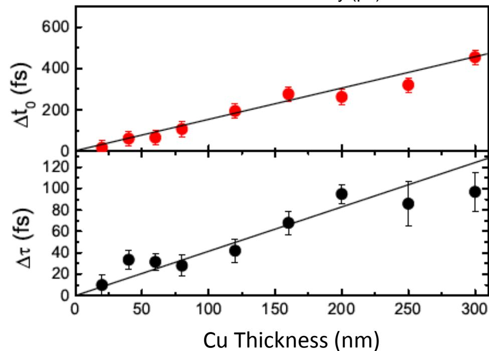
Linear variation of  $\Delta t_0$  up to 300 nm / Hot electrons velocity of  $0.7 \times 10^6$  m/s
