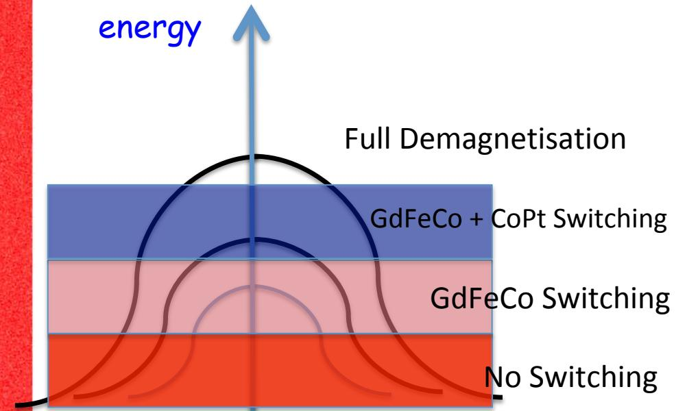
Pump energy dependence of radius of the domain can be explained by the Gaussian distribution of the pump laser
