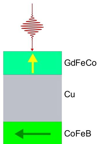
Recent experimental study demonstrated that spin-polarization of spin current generated by GdFeCo is parallel to Gd
