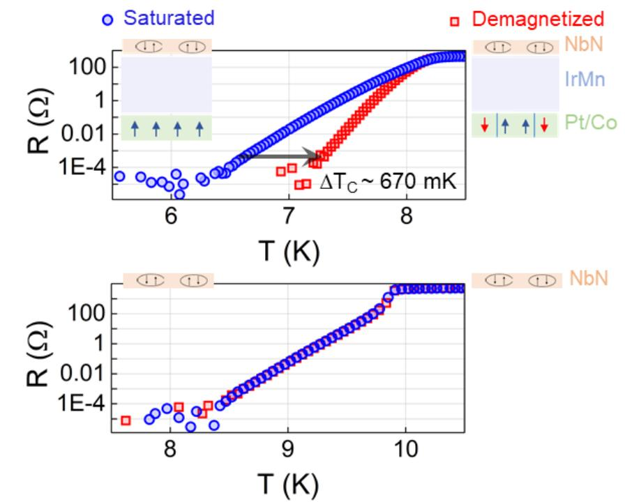
$[\text{Pt}/\text{Co}]_{x15}/\text{IrMn}/\text{NbN}$  stacks with  $\xi_s(T_c) \sim d \sim t_s \sim t_F \sim 15 \text{ nm} < D \sim 50 \text{ nm}$
