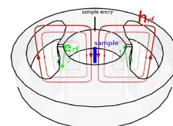
3 loop - 2 gap resonator  $\sim$  mode  $TE_{102}$
