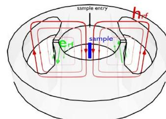
3 loop - 2 gap resonator  $\sim$  mode  $TE_{102}$
