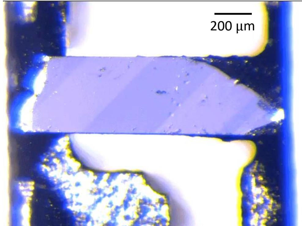
Sample mounted in a uniaxial pressure cell and domains identified using standard polarised light microscopy
