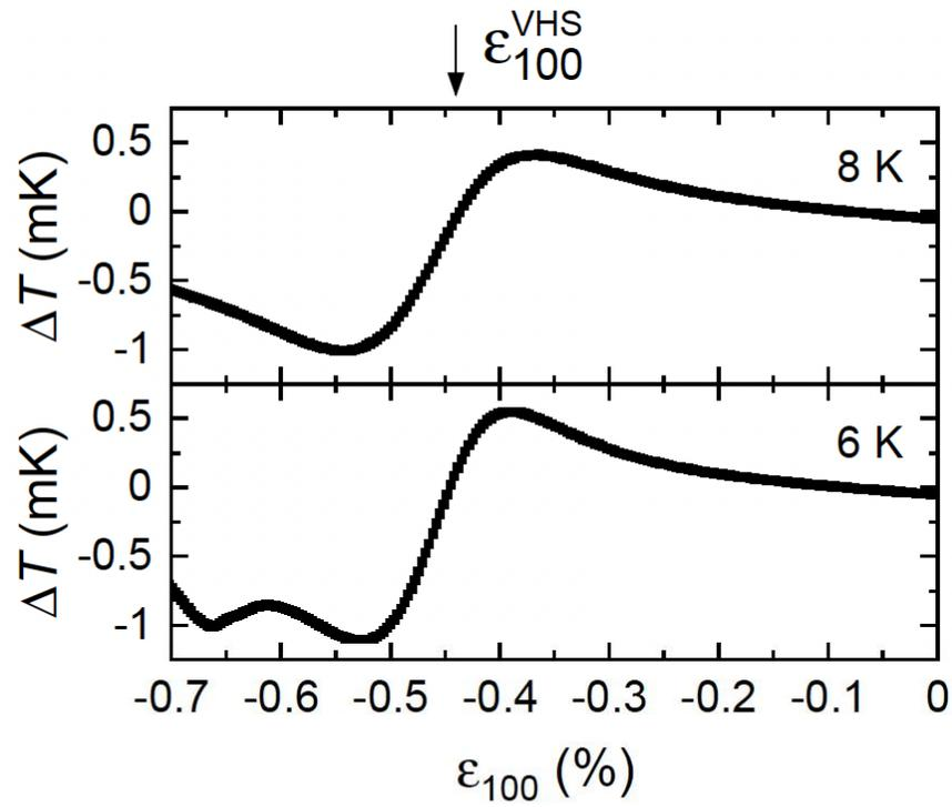
Due to high thermal precision  $\sim \mu\text{K}/\text{Hz}^{1/2}$ , easily resolve elastocaloric signal in  $\text{Sr}_2\text{RuO}_4$  for ppm applied a.c. strains superimposed on d.c. compression
