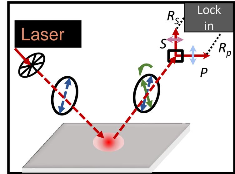
Transfer cell to Montana Instruments optical cryostat and re-measure birefringence using laser setup
