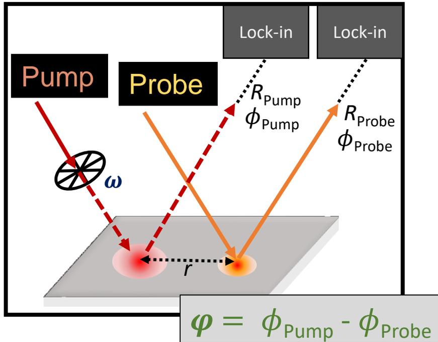
Idea: use pump laser to apply an a.c. heat source
