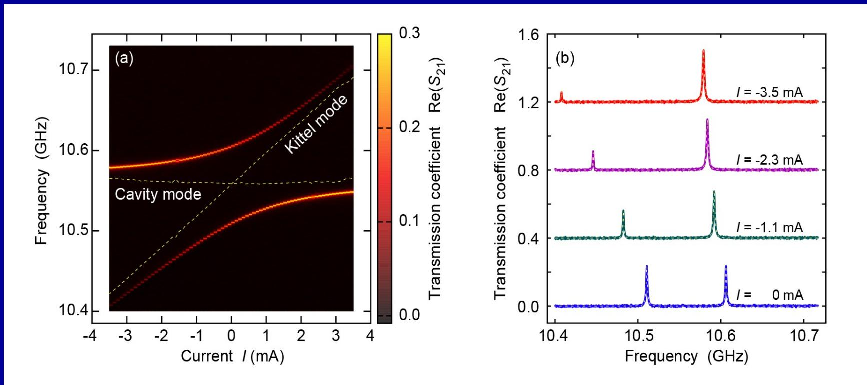
Normal mode splitting between a magnon (YIG) and a cavity mode
