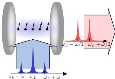
Single diss. cavity mode coupled to collective spin
