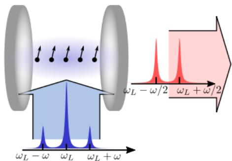
Cavity photons mediate time-periodic interactions between the atoms
