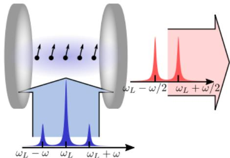
Cavity photons mediate time-periodic interactions between the atoms
