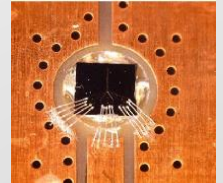
Wired bonded custom chips to single mode microwave PCB
