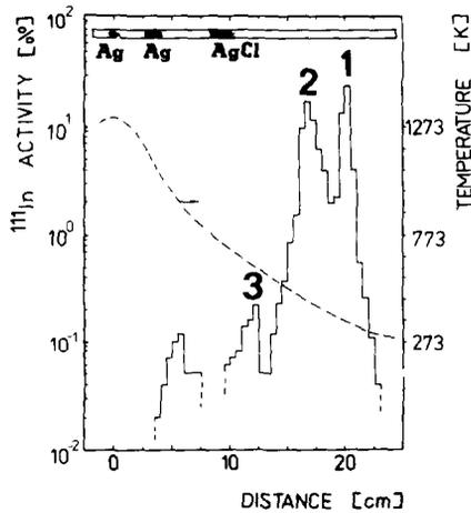
Fig. 2. Thermo-chromatogram of the indium chlorides, evaporated into the gas phase from the irradiated silver experimental time: 1 h,  $p_{\text{HCl}}/p_{\text{H}_2\text{O}} = 0.1$ , total pressure: 6.67 Pa.
