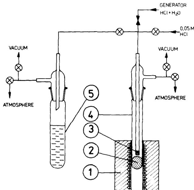
Fig. 3. Remotely controlled version of the method for the high temperature extraction of  $^{111}\text{In}$  from silver. 1—electric furnace, 2—silver sample, 3—quartz filter, 4—quartz device for  $^{111}\text{In}$ -release, 5— $^{111}\text{In}$ -container.
