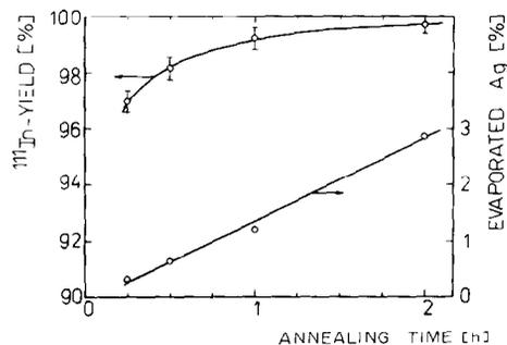
Fig. 1. Dependence of the  $^{111}\text{In}$ -extraction and of silver evaporation on time.
