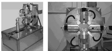
Fig. 1. Photograph of the YAP-(S)PET scanner (left) and zoom of the four rotating heads (right).
