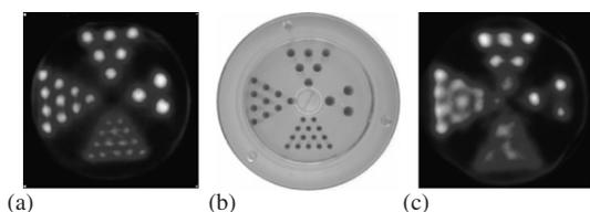
Fig. 2. From the right moving anti-clock wise we have 3.0, 2.5, 2.0 and 1 mm diameter holes. (a) PET image obtained with EM algorithm (50–850 keV). (b) Photograph of the Derenzo phantom. (c) Reconstructed image in SPECT: EM algorithm (140–250 keV).
