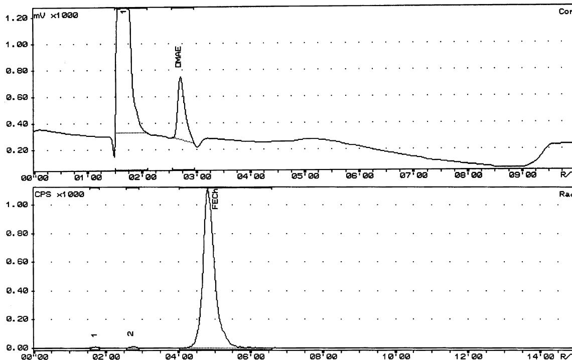
**Figure 5.** Typical radiochromatogram of the quality control of  $[^{18}\text{F}]$ FECh using ion exchange chromatography.
