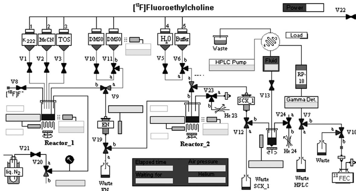
Figure 4. Schematic diagram of the automated synthesis module.
