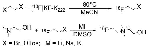
**Figure 2.** Synthesis of  $[^{18}\text{F}]$ fluoroethylcholine.
