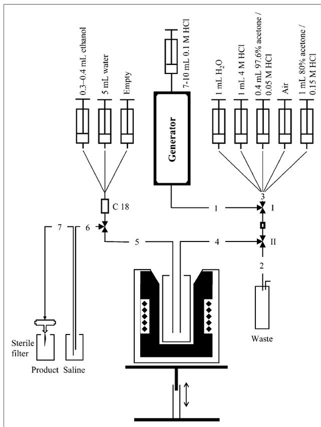
**FIGURE 1.** Scheme (top) and post-processing of  $^{68}\text{Ga}$ -eluates and generator-associated syntheses of  $^{68}\text{Ga}$ -labeled compounds (e.g., labeling and product purification for DOTATOC as a proof-of-principle precursor).
