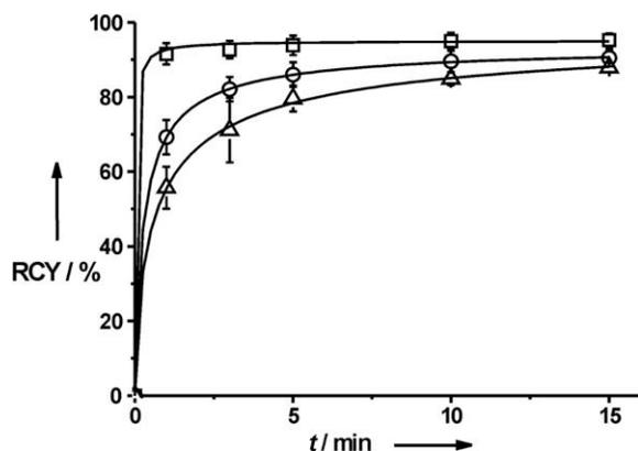
**Figure 1.** Radiochemical yields (RCY) of **10** by labeling of DO<sub>2</sub>A-(OBu-L-tyr)<sub>2</sub> (**9**) with <sup>68</sup>Ga at three different temperatures (90 °C (squares), 70 °C (circles), 50 °C (triangles)) in aqueous solution. Labeling yields are given as mean values (%) ± standard deviation.
