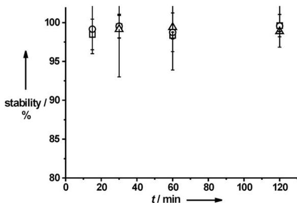
**Figure 2.** Challenge experiment of [<sup>68</sup>Ga]Ga-DO<sub>2</sub>A-(OBu-L-tyr)<sub>2</sub> with 10 ml of DTPA in two concentrations (1 mmol, 750-fold excess; squares; 1 μmol, 0.75 equiv, circles) and 5 ml transferrin solution (1 mmol, 375-fold excess, triangles) at 37 °C over 120 min (*n* = 3). Stability values were expressed as mean values of intact tracer (%) ± one standard deviation.
