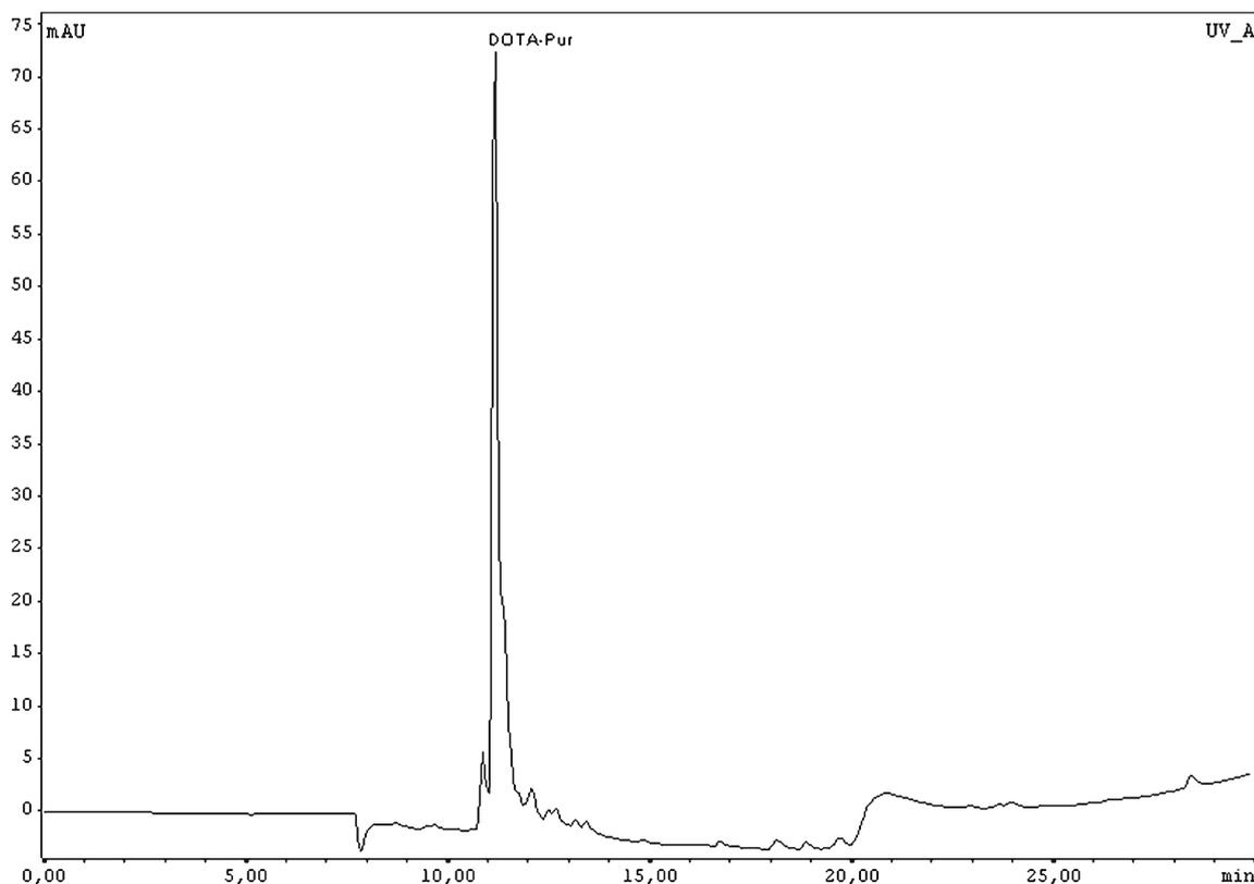
**Fig. 2.** HPLC-chromatogram of DOTA-Pur—solvent A, 0.1 % trifluoroacetic acid (TFA)/H<sub>2</sub>O; solvent B, 0.1 % TFA/acetonitrile; gradient elution, 0 min, 80 % B—20 % C; 30 min, 60 % B—40 % C.
