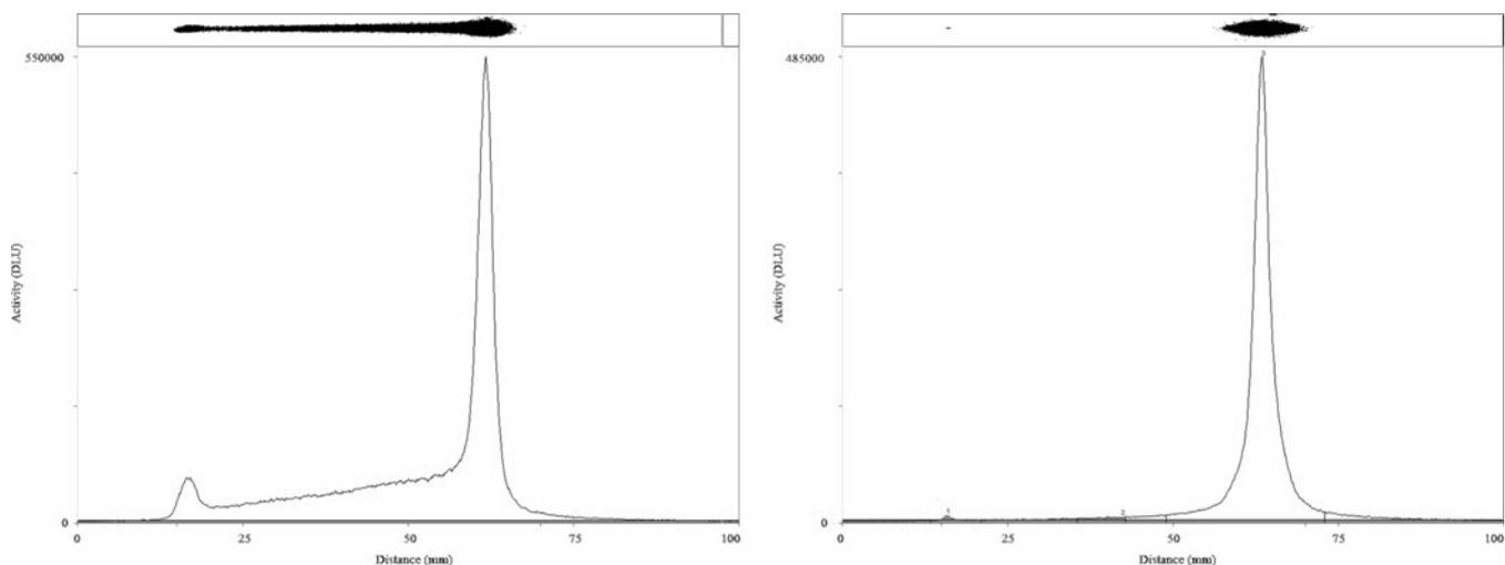
**Fig. 3.** Instant thin-layer chromatograms (iTLC) of reaction mixture and purified product in 0.9 % saline solution; radiochemical purity after purification  $\geq 97$  %.
