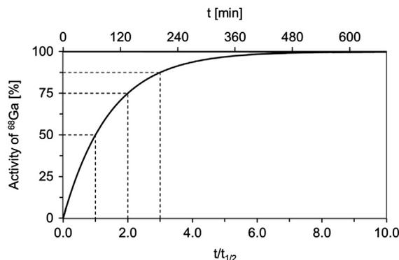
Fig. 2. Kinetics of the secular equilibrium of the  $^{68}\text{Ge}/^{68}\text{Ga}$  radionuclide generator for  $A_{\text{Ga}}^0 = 25\%$  and  $50\%$  of the saturation (equilibrium) activity of  $^{68}\text{Ga}$  are being generated after 28.10 and 67.71 min.
