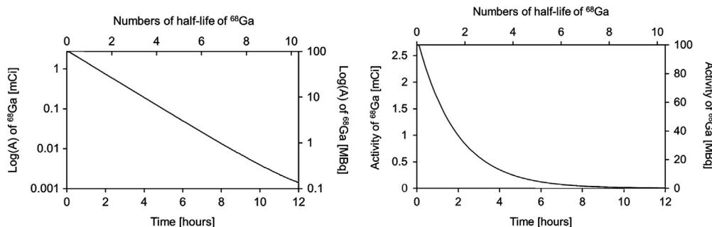
Fig. 1. Decay of initially eluted 27 mCi of  $^{68}\text{Ga}$  in terms of real time after elution (lower x-axis) and multiples of half-life of  $^{68}\text{Ga}$  (upper x-axis), with logarithmic (LOG) or linear scale (LIN) of activity.
