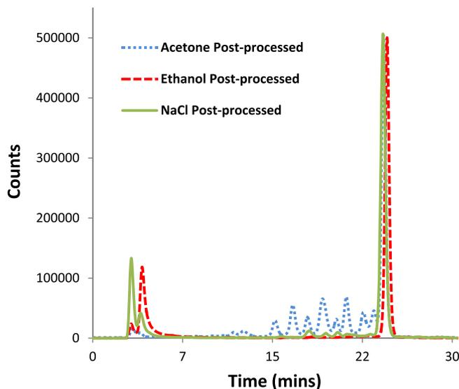
Fig. 2. HPLC chromatograms of  $^{68}\text{Ga}$ -DOTATOC ( $R_t=24$  min) 45 min after preparation using  $^{68}\text{Ga}$  obtained using each of the three different post-processing methods. Count values have been normalised for clarity. Unreacted  $^{68}\text{Ga}$  from the labelling solution elutes with a retention time of 3–4 min. Radiolytic decomposition is indicated by impurities eluting between 15 and 24 min.
