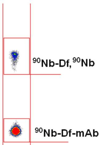
**Fig. 2.** ITLC image of quantification of labeling efficiency for  $^{90}\text{Nb}$ -Df-bevacizumab after 60 min of reaction. Stationary phase: paper impregnated chromatography strip, mobile: phase, 0.02 M citrate buffer (pH 5.0).
