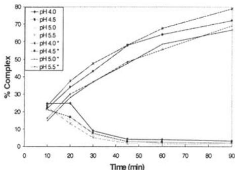
Fig. 2. Effect of pH on gluconate complexation of  $^{188}\text{Re}$  at 0.2 M sodium acetate at 37°C. \*under nitrogen.
