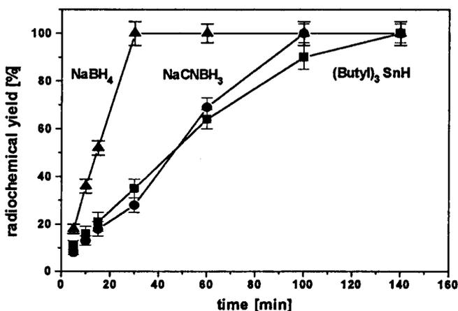
Fig. 1: Influence of the reduction agent on the radiochemical yield of n.c.a. 3- $^{18}\text{F}$ fluorotoluene (based on 3- $^{18}\text{F}$ fluoro-2-iodotoluene). Reaction conditions : [hydro-deiodination agent] 35 mmol/L, uv-activation ( $\lambda = 254\text{nm}$ ), room temperature, 1 mL acetonitrile.
