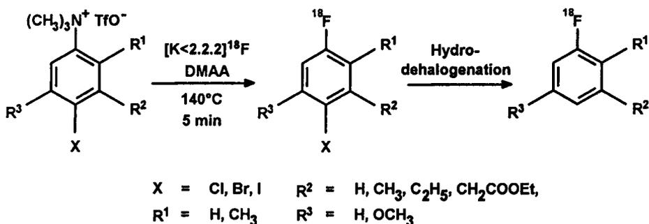
**Scheme 1:** Synthesis of 2- and 3-[<sup>18</sup>F]fluoroalkylarenes via halogen activation of the aromatic ring
