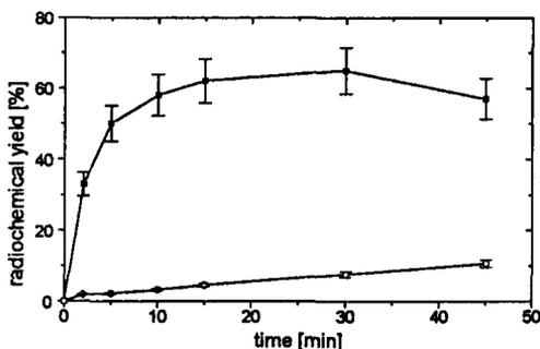
Fig. 1: RCY of [<sup>131</sup>I]MeOBH (■) and the corresponding acid (□) as function of time (90%TFA, Iodogen, 60°C, 32 mM OMeBH)
