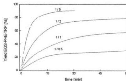
Fig. 2: Kinetics of the reaction EGS + PHE-TRP as a function of educt ratios.
