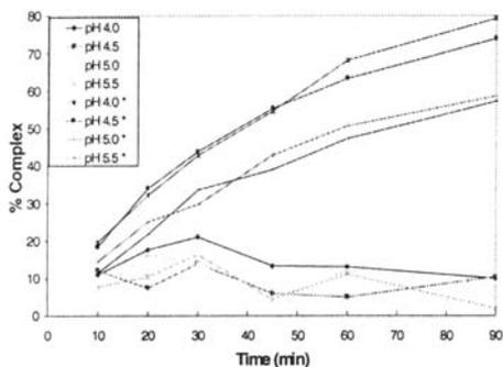
Fig. 3. Effect of pH on citrate complexation of  $^{188}\text{Re}$  at 0.2 M sodium acetate at 37°C. \*under nitrogen.
