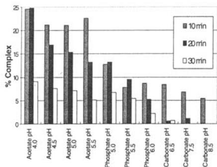
Fig. 1. Effect of pH on gluconate complexation of  $^{188}\text{Re}$  in various buffers<sup>a</sup> at 37°C in the absence of nitrogen.
