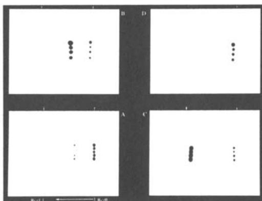
**FIGURE 2:** TLC-radiochromatograms of reaction mixtures during the radiosynthesis of [F-18]FLT.
