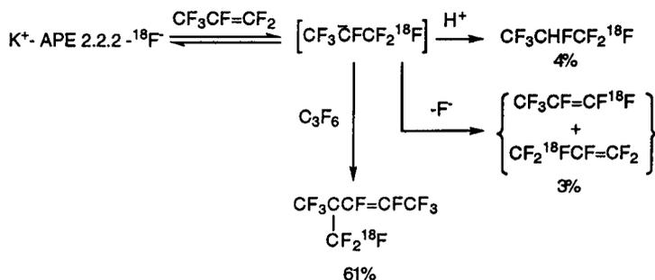
Scheme 3: The reaction of  $\text{K}^+\text{-APE 2.2.2-}^{18}\text{F}$ fluoride with hexafluoropropene.
