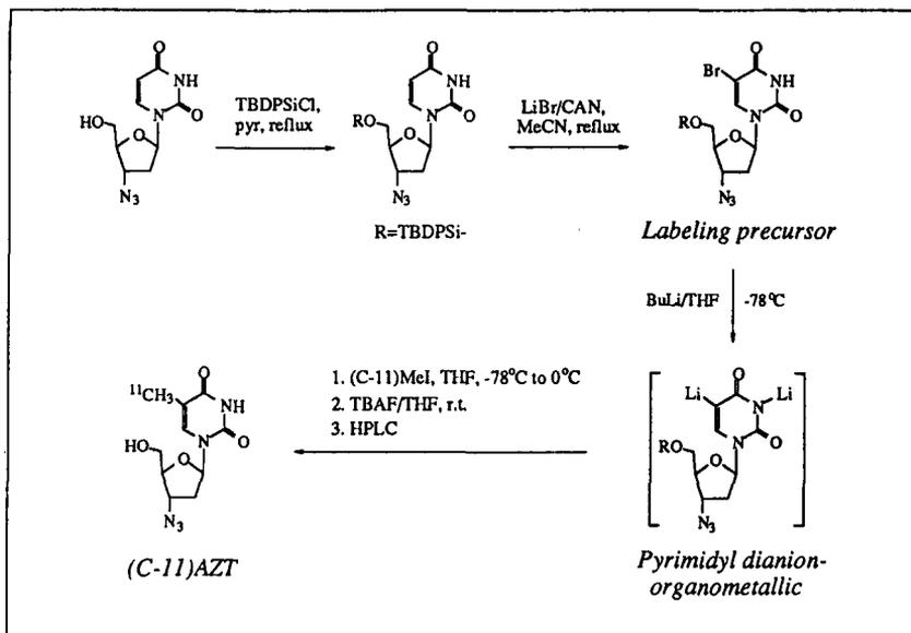
Figure 1: Precursor synthesis and labeling chemistry for (C-11)AZT.
