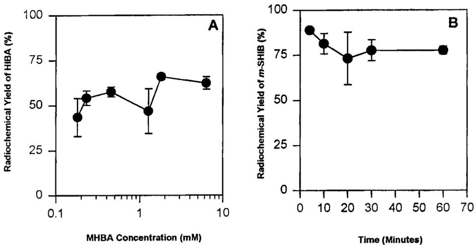
Figure 1. A) Dependence of radiochemical yield of [<sup>131</sup>I]HIBA production on the concentration of *meta*-hydroxybenzoic acid. B) Yield as a function of time in the formation of *m*[<sup>131</sup>I]SHIB.
