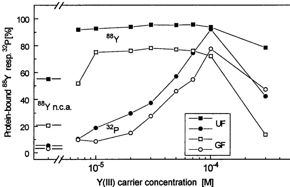
Fig. 1 Percentage of  $^{88}\text{Y}(\text{III})$  and  $^{32}\text{P}$ phosphate bound to HSA vs. Y(III) carrier concentration (GF = gel filtration, UF = ultrafiltration)
