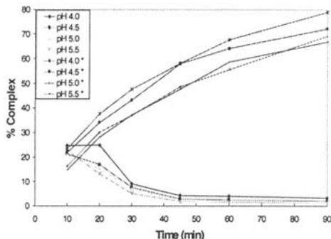
Fig. 2. Effect of pH on gluconate complexation of  $^{188}\text{Re}$  in 0.2 M sodium acetate at 37°C. \*under nitrogen.
