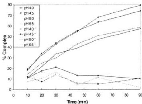
Fig. 3. Effect of pH on citrate complexation of  $^{188}\text{Re}$  in 0.2 M sodium acetate at 37°C. \*under nitrogen.
