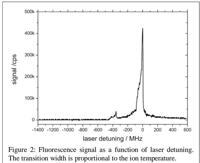
Fluorescence was detected using a channel-photomultiplier, with the detection setup designed at Münster University. Its high detection efficiency and low dark count rate allowed detection of even a single trapped ion. This offered a unique opportunity to detect ions non-destructively, either by means of fluorescence detection or by electronic pick-up of the induced image charge.
