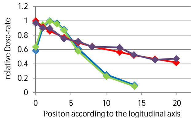
Figure 1: Dose response  $R_{\text{Alanine}}$  on the longitudinal axis of the phantoms (measured: blue – FiR1, red –TRIGA; calculated: green – FiR1, purple – TRIGA)
