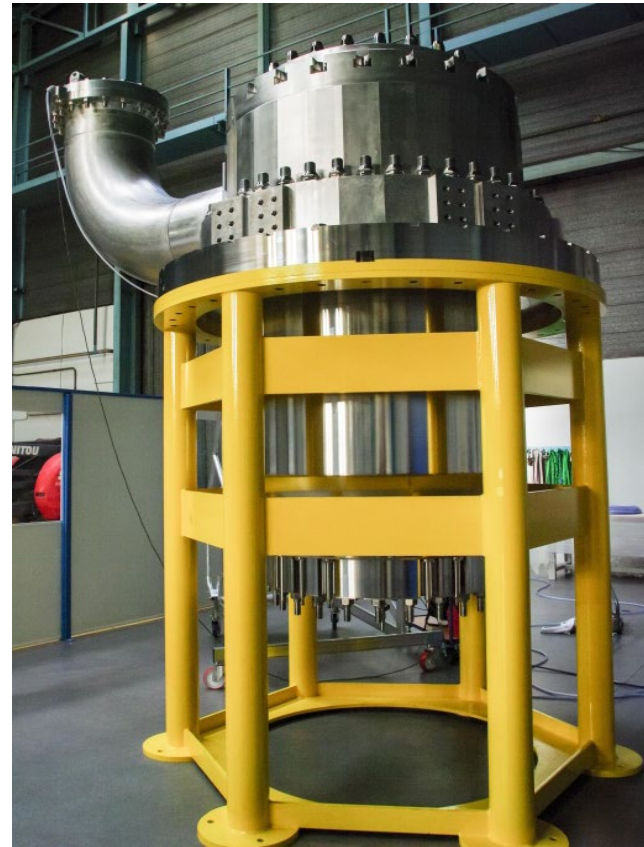
Primary water box and plug
