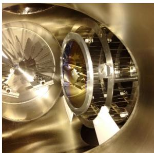
The uranium-233 source (large disk in center of image) produced at the Johannes Gutenberg University Mainz, Germany, mounted inside the experimental apparatus at the Ludwigs-Maximilian-University Munich, Germany. Components of the setup are reflected in the surface of the source.
