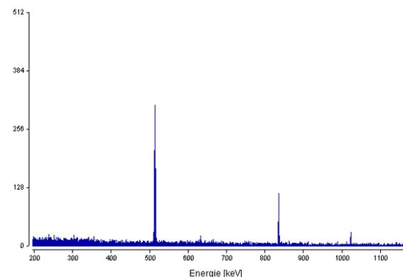
Fig.2:  $\gamma$ -spectrum of nca  $^{72}\text{As}$  after elution, characteristic  $\gamma$ -lines: 511 keV (176 %), 834 keV (80 %), 1023 keV (Sum-Peak)
