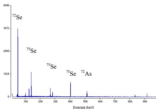
Fig.1:  $\gamma$ -spectrum of the  $^{72}\text{Se}/^{72}\text{As}$  isotope generator before elution (characteristic emissions of  $^{75}\text{Se}$ , side-product of cyclotron production of  $^{72}\text{Se}$ , are also observed)
