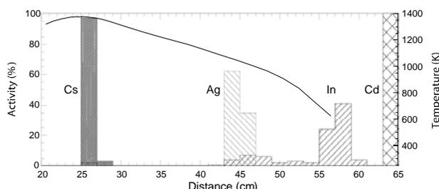
Fig. 2: The deposition of Ag, Cd, In and Cs on quartz surfaces.
