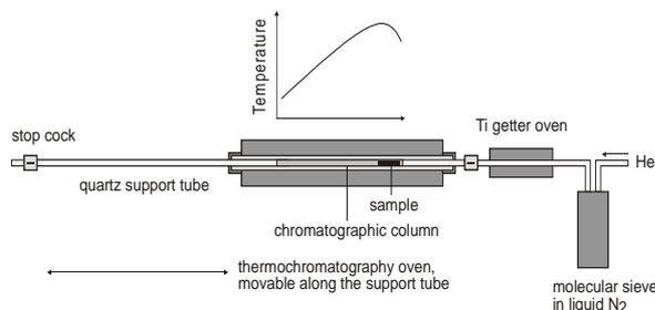
Fig. 1: Setup of the TC experiment at the TRIGA Mainz.
