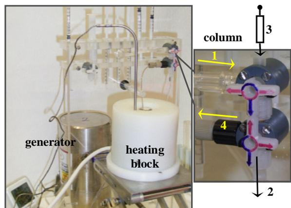
Fig. 1. Equipment for labelling of DOTATOC with generator-produced <sup>68</sup>Ga; to the right the micro-chromatography column.
