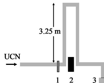
**Fig.1:** Sketch of the gravitational spectrometer; 1: vacuum shutter; 2: 10 cm borated polyethylene; 3: UCN detector with 0.1 mm aluminium entrance window. The detector was shielded against background in a box of 10 cm borated polyethylene (not shown).
