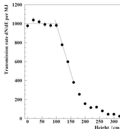
**Fig. 2:** Data taken with the gravitational spectrometer. The UCN transmission rates per megajoule of the reactor power are plotted against the vertical height of the gravitational spectrometer. The two lines represent the fit to the data, see text.
