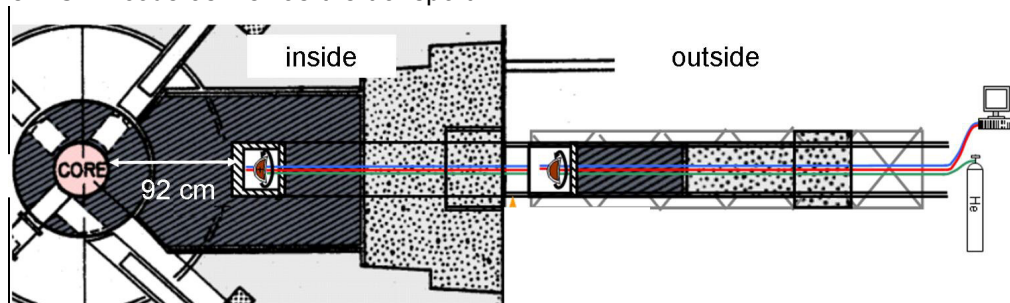
Fig.2: Planned modification of the irradiation channel of the thermal column. The image shows the transportation system for the organ, the gamma shielding is not included in the picture
