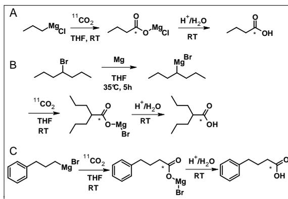
**Fig. 1:** Radiosynthesis of [ $^{11}\text{C}$ ]BA (A), [ $^{11}\text{C}$ ]VPA (B) and [ $^{11}\text{C}$ ]PBA (C).
