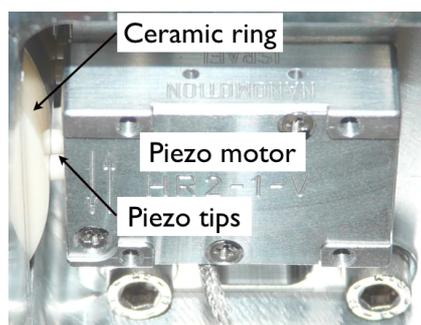
Figure 3: The piezo actuators of the UCN switch.
