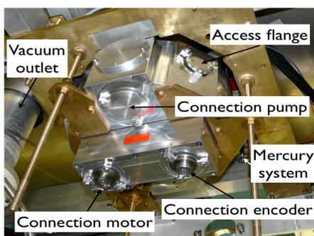
Figure 1: UCN switch underneath the nEDM experiment.
