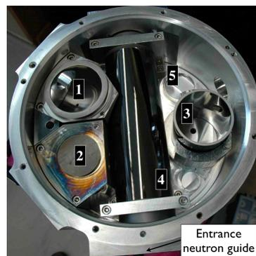
Figure 2: Interior parts of the UCN switch.
